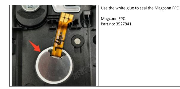
Replacement of Speaker Disassembly the speaker
