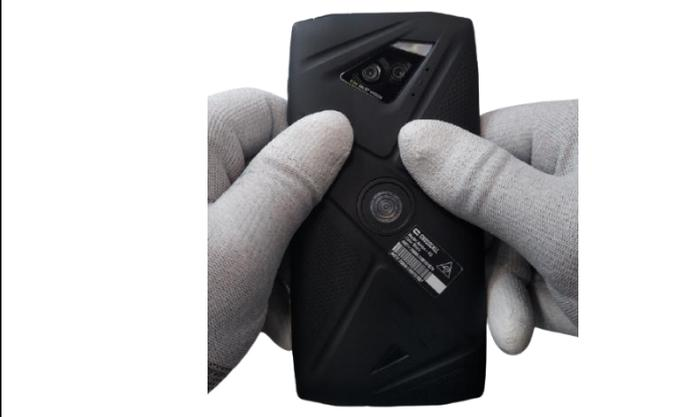
A photograph showing a pair of gloved hands holding the smartphone. The battery cover is now fully attached to the back of the phone, covering the camera and flash area.                         | <p>Presser l'ensemble du cache batterie pour plaquer l'adhésif entre les cosmétiques.</p> |
