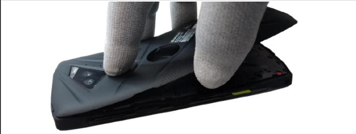
A close-up photograph showing a pair of gloved hands positioning the black battery cover onto the back of a smartphone. The cover is being aligned with the camera and flash area.                | <p>Positionner le cache batterie sur la cosmétique arrière.</p>                           |
