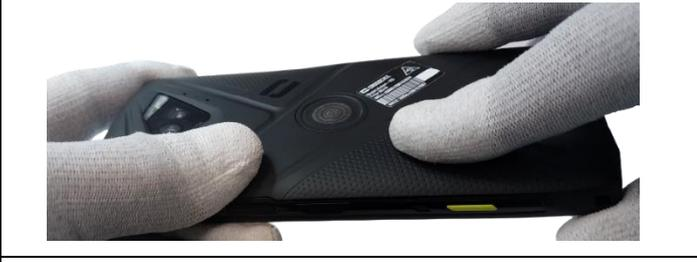
A close-up photograph showing a pair of gloved hands pressing the battery cover onto the back of the smartphone. The hands are applying pressure to the edges of the cover to clip it into place. | <p>Presser le contour du cache pour le clipser.</p>                                       |
