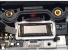
Use the flat-nose pliers to remove the earpiece. Be careful not to damage the membrane on the cosmetic during this operation.
