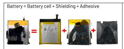
The shielding and adhesive can be peeled off and reused on a new battery cell.
