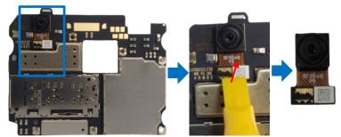
Also remove the front camera using the same tool.
