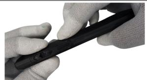
Press around the edge of the cover to clip it into place.
