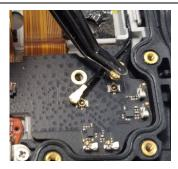
Remove the vibrator by inserting a flat pair of tweezers from underneath and disconnect the 2 coaxial cables.
