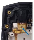
Insert the jack connector in the direction indicated by the green arrow.
