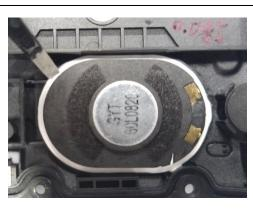
Use the flat-nose pliers to remove the speaker. Be careful not to damage the membrane on the cosmetics during this operation.
