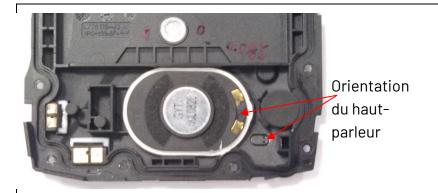
Place the speaker in its compartment, in the direction shown in the photo. The contacts should face to the right as indicated by the indicator on the cosmetic.
