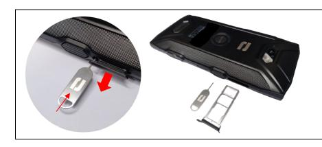
Extract the SIM drawer by inserting the extractor into the drawer hole.
