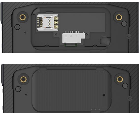
After installing the cards correctly, press the seal cover tightly.
