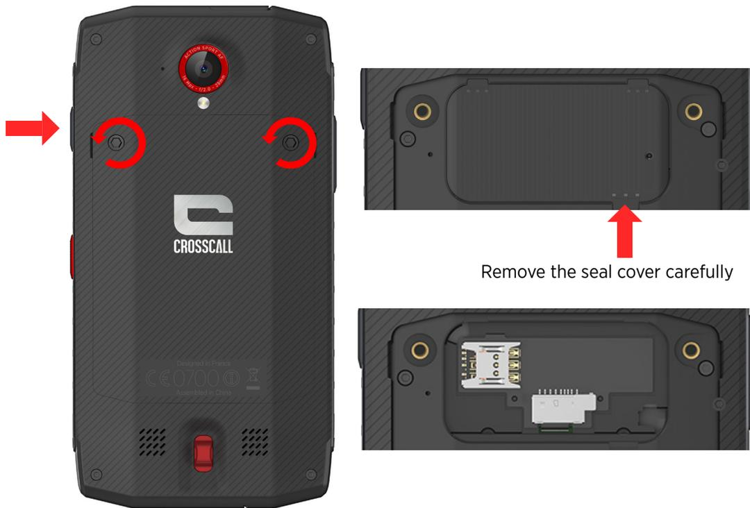
**Warning:** Take care about the antenna when you remove the seal cover. Do not use tool to remove the seal cover to not damage the rubber seal.
