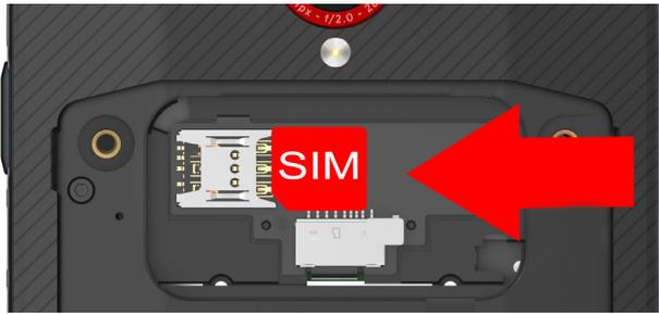
First insert Nano SIM (4FF) card into the phone as shown (contacts face down)
