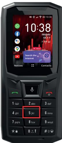
From the Home screen, press and hold the 5 key to enable/disable connection sharing (tethering).
