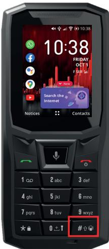
Press and hold the # key to switch from vibrate to ring mode, and vice versa.
