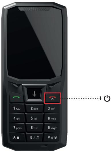
Press and hold the phone's On/Off button and wait a few seconds until the display turns on.
